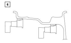
Slide out the gauge on the LH side, at the point where a weight is to be fitted. Wait until the symbol shown in Figure 5d is displayed. Pull it out further towards the right plane and wait until the symbol shown in Figure 6A is displayed. The wheel balancer automatically identifi es ALU S mode.
