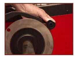
Place the round part of the gauge terminal on the flange as shown in the figure and press
