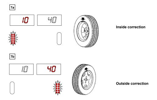
After performing a balancing spin, the amounts of unbalance are shown on the digital readouts. The illuminated LEDs 3 and 4 indicate the correct angular position of the wheel to mount the counterweights (12 o'clock).
