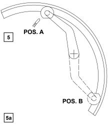
For clamp weights, use the gauge in the top position A. For adhesive weights, use the gauge as preferred in top position A or bottom position B.
