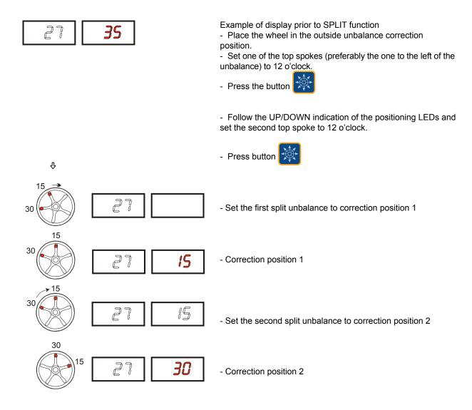
**N.B.:** If error 24 is displayed, repeat the SPLIT function ensuring that the minimum distance between the spokes is greater than 18 degrees. If error 25 is displayed, repeat the split function ensuring that the maximum distance between the spikes is smaller than 120 degrees.
