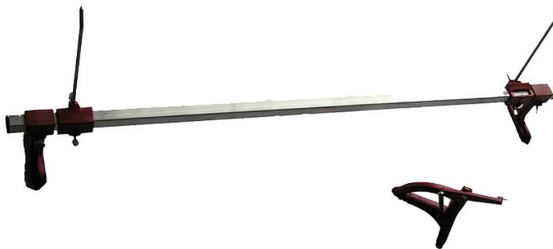
It is preferable to check toe with the wheels on Turntables since wheels are permitted to move freely during adjustments. **The Locking Pins should not be in place.** Work the steering wheel back and forth rapidly several times to settle the wheels in their normal driving position.
