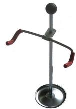
Toe-In should be checked and adjusted on a level floor or with the front wheels on the Turntables and the lock pins removed. The wheels should first be spread apart at the front to compensate for any looseness, using the Front Wheel Spreader.
